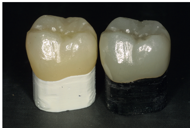
Figure 2. Cubic zirconia UT 1.5-mm crowns placed on black and white dies used as backgrounds in CR measurements. Note great color differences generated by dark background, giving measurements of material's high translucency. Panavia V5 clinical evaluation paste served as optical connection between dies and crowns. CR, contrast ratio; UT 1.5, Katana zirconia ultra translucent multi-layered EA2 Lot DLVUQ.
