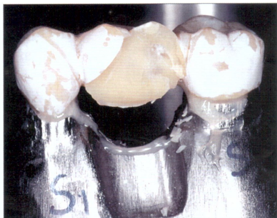
Fig 1 Targis and Vectris fractures of an aged specimen. Many cracks occurred during the flexure test. Note the dull white color of the altered resin composite surface.
